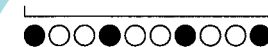
Cross section of lighting arrangement with black lights in number 1, 4, 7 and 10 positions.
