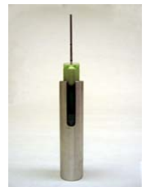
Fig.4 Measure the falling time between two markings on the extension bar attached to the needle.
