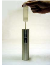
Fig.1 Slide the syringe into the viscometer main body.
