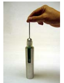
Fig.3 Insert the needle into the syringe until the top of the needle reaches the top of the syringe and then drop the needle.
