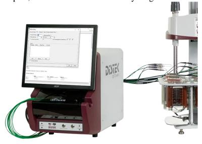
**Run Automation for Complete Systems:** For systems comprised of Distek baths equipped with a Dosage Auto-Dropper (DDS) option, complete run automation is now possible. Technicians can initiate the process with a simple start command. The software autonomously manages agitation and heating, dosage dropping at optimal media temperatures, and data collection, culminating in the automatic generation, storage, and optionally printing of final reports.
