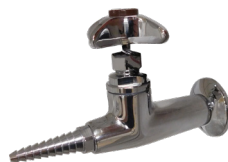
Single Keycock Single flange mounted needle valve, keycock with integral flange and shank connection. Epoxy coated brass. 3/8" NPT with lock nut. Single Cat. No. 50025 Double Cat. No. 50125
