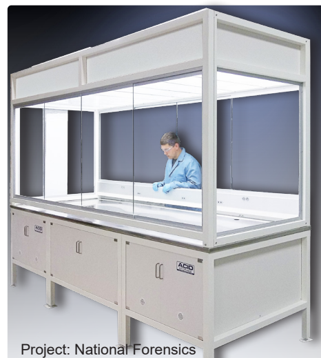
Project: National Forensics & Coroners Complex, Canada EnviroMax enclosure, unitized 120" wide X 36" deep X 48" high, with custom acid storage cabinets
