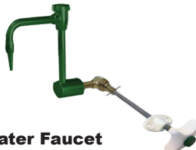
DI Faucet Pure water 6" swivel tin-lined goose neck. Epoxy coated brass. Cat. No. 50022
